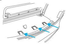
Tether anchorage hardware kits (part number 613D20) including instructions, may be obtained at no charge from any Ford or Lincoln-Mercury dealer. All vehicles built for sale in Canada include a tether anchor hardware kit.
